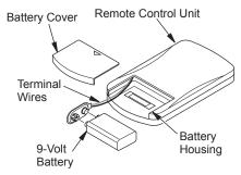
Figure 40 - Installing Battery in Hand-Held Remote Control Unit
